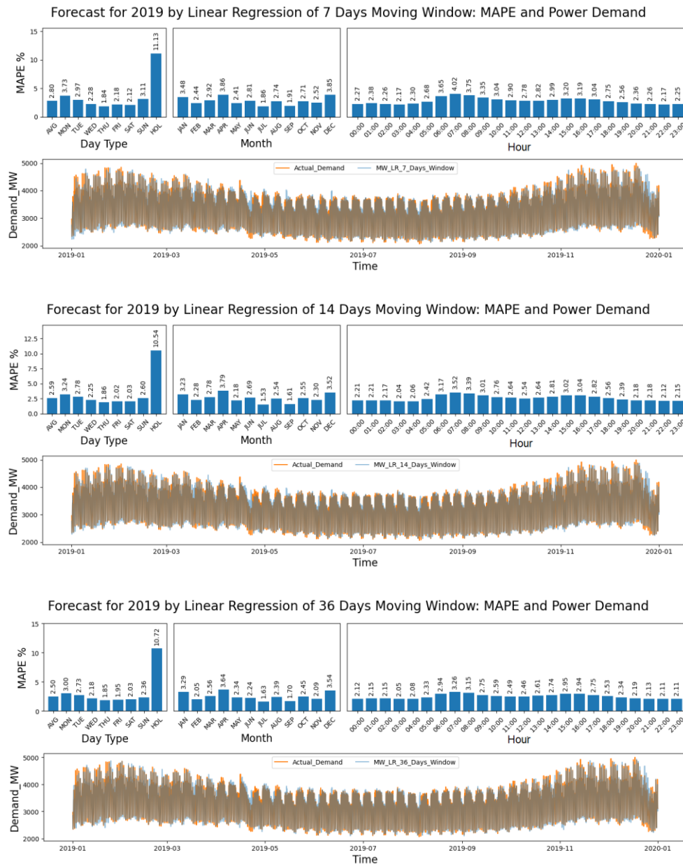
Figure 7.4. Forecast of power demand for year 2019 by linear regression for moving window size of 7, 14 and 35 days.
