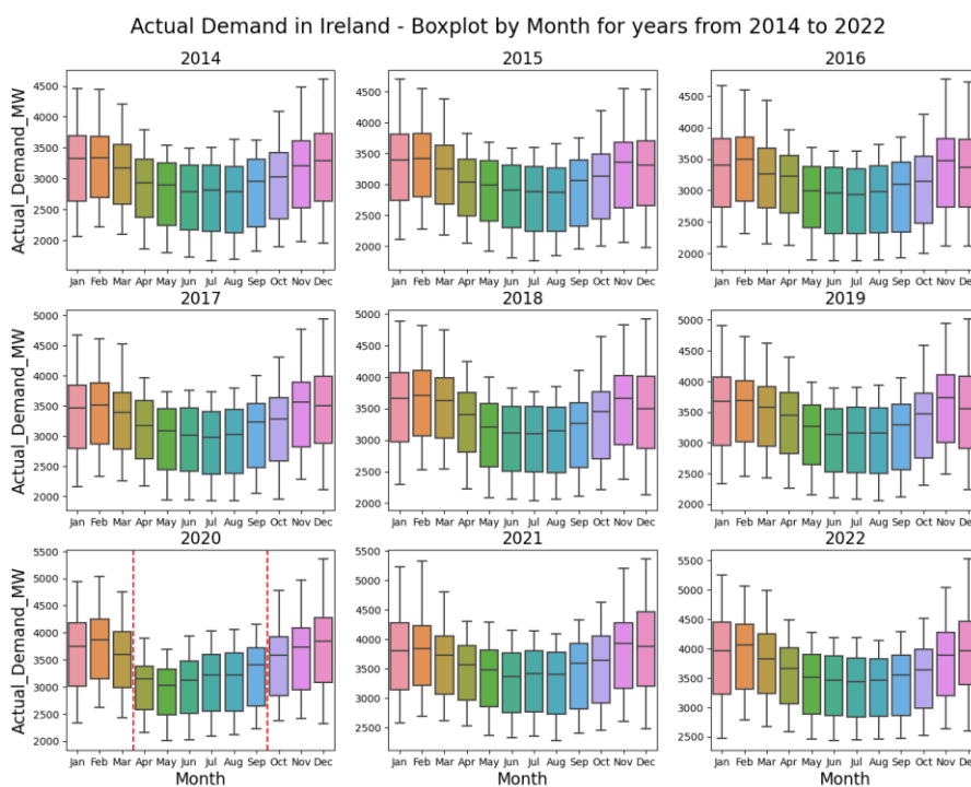
Figure 5.12. Monthly boxplots of power demand in Ireland by years. Covid-19 lockdown period marked as dashed red lines.
