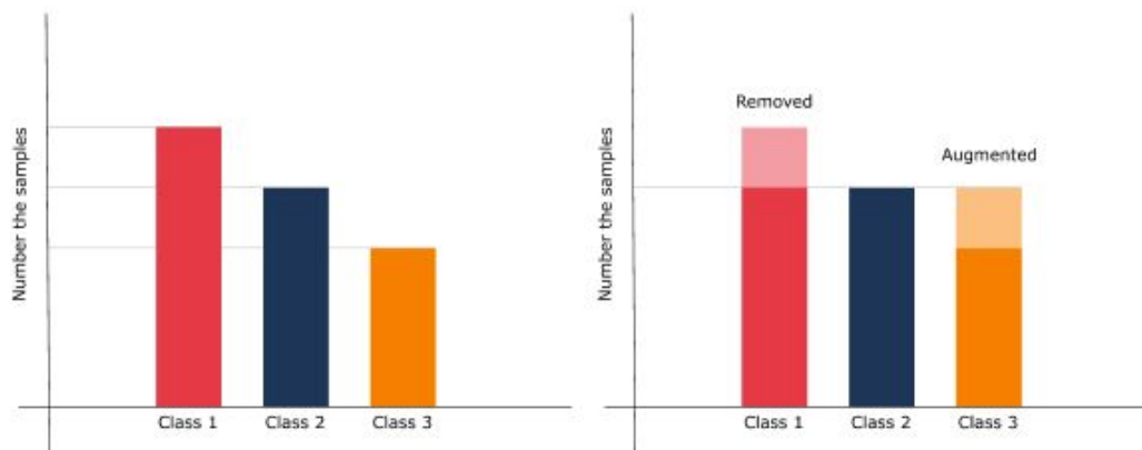
Image 9 - In the example above, a generic dataset has three unbalanced classes, which are manipulated to contain roughly the same number of samples utilised
