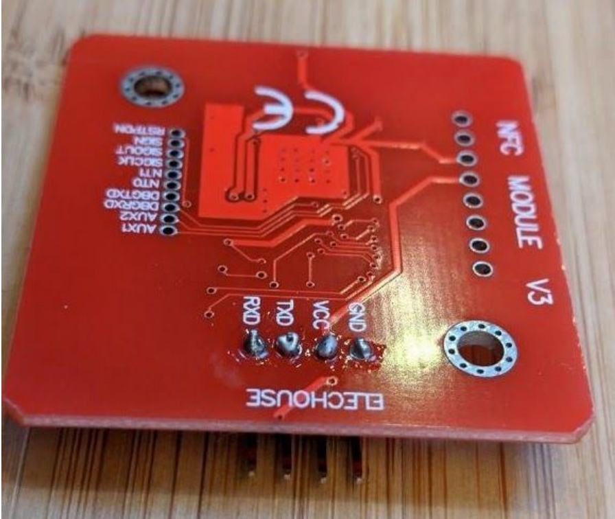
Figure 8.1.3: NFC-Reader after soldering
