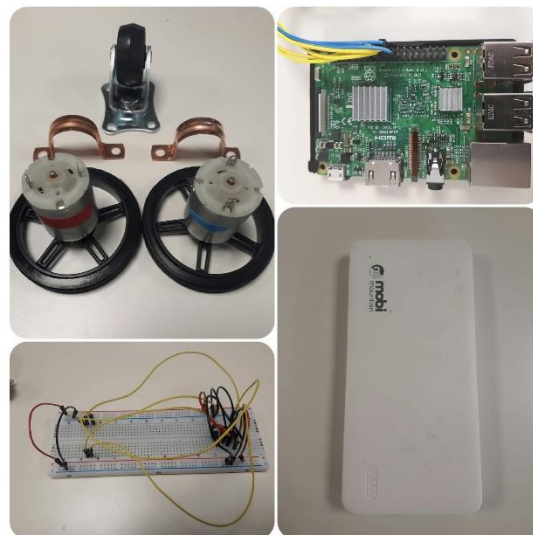
Figure 23: Left top, Swivel wheel, motors, copper clamps and wheels. Right top, Raspberry Pi. Left Bottom, Breadboard with chip L293D. Right Bottom: Battery bank 10000mA.
